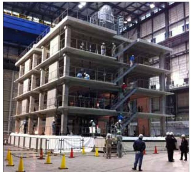
RC structures being tested side-by-side (photo: Jack Moehle).
